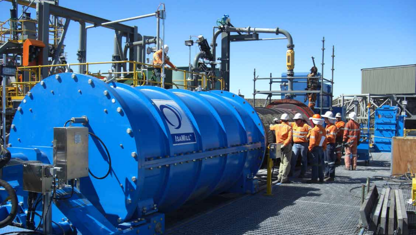
IsaMill uses a ceramic medium which wears ten times slower than steel
