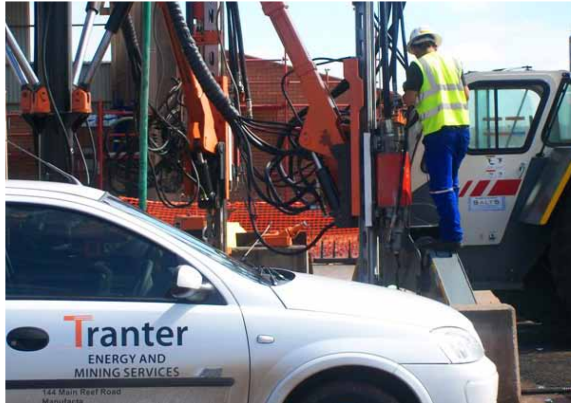
Employee testing S140 on shaft sinking jumbo
