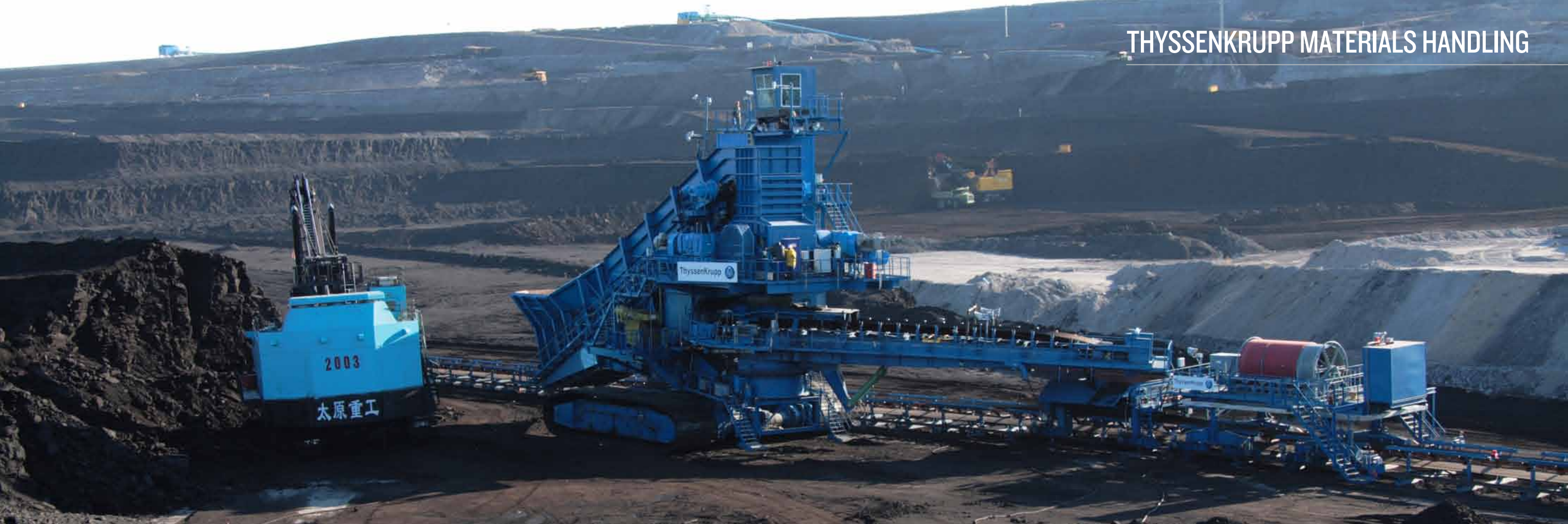
Mobile crushing plant
