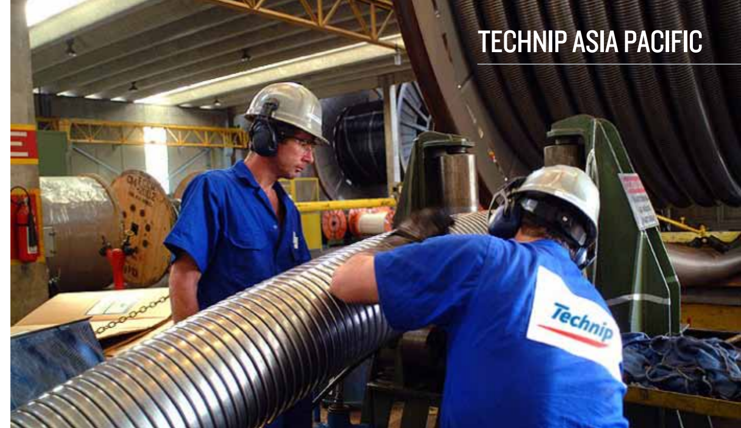
The production of flexible pipes at Technip’s plant
