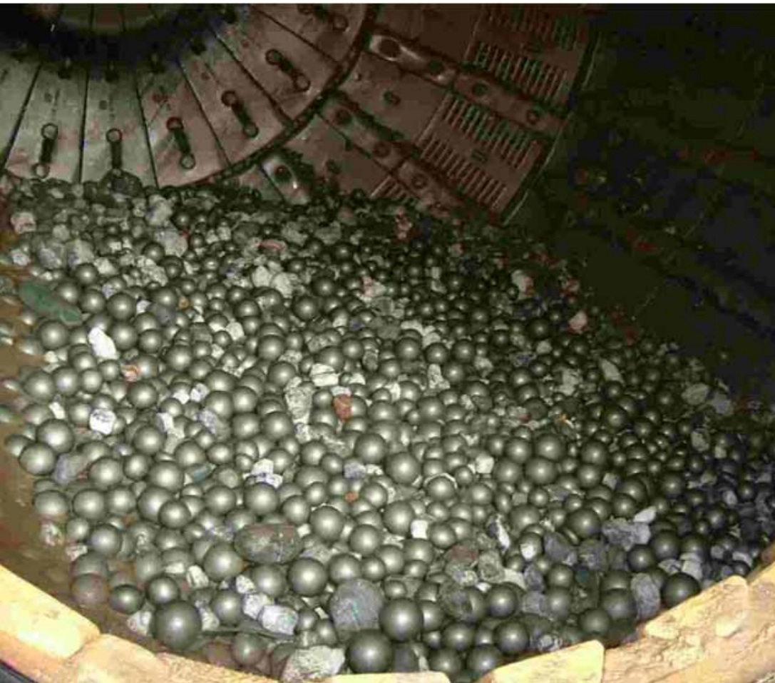
125mm Sino-4 grinding balls in a 6.5m SAG mill
