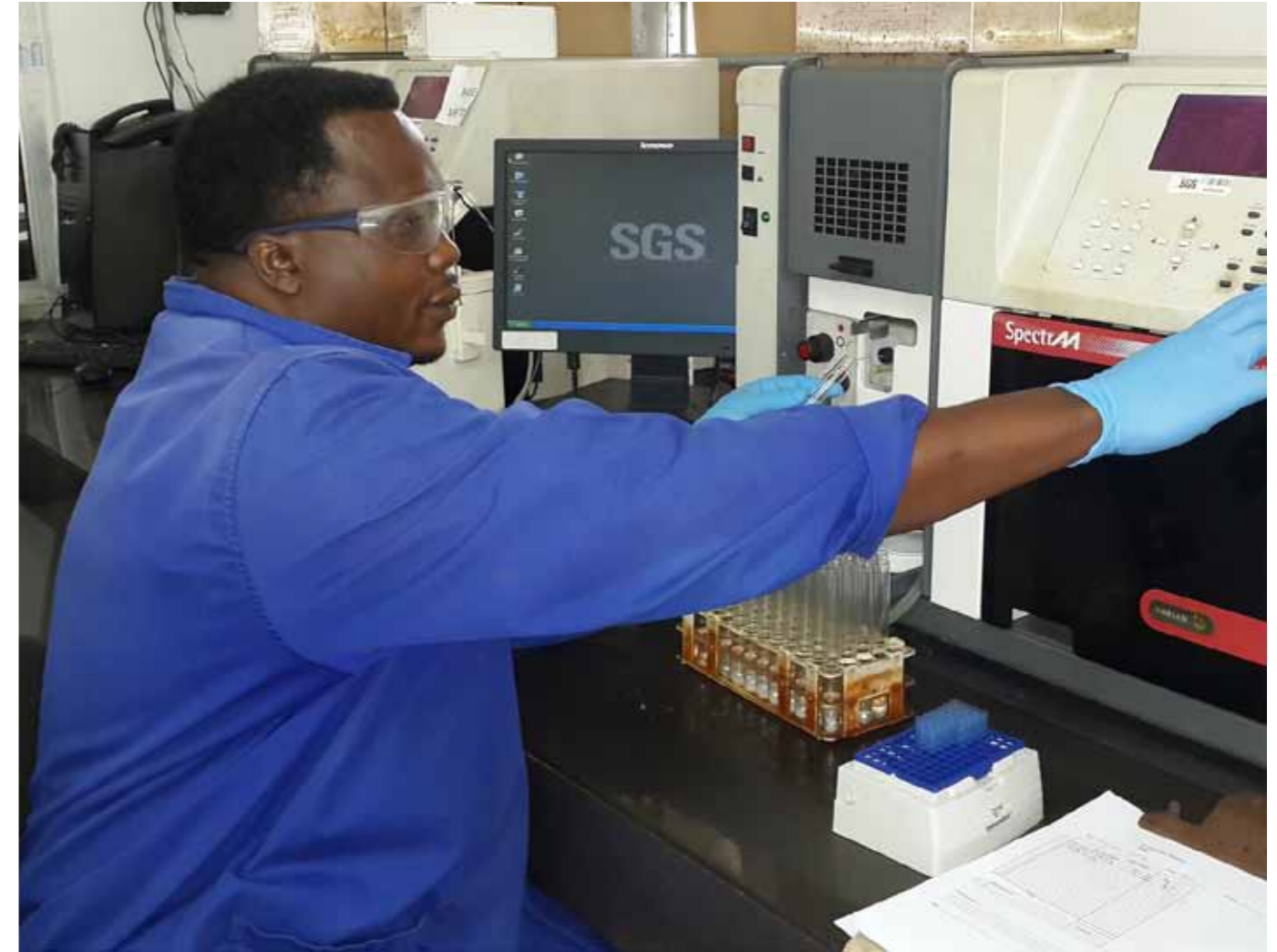
Chemist on AAS for determination of precious and base metals
