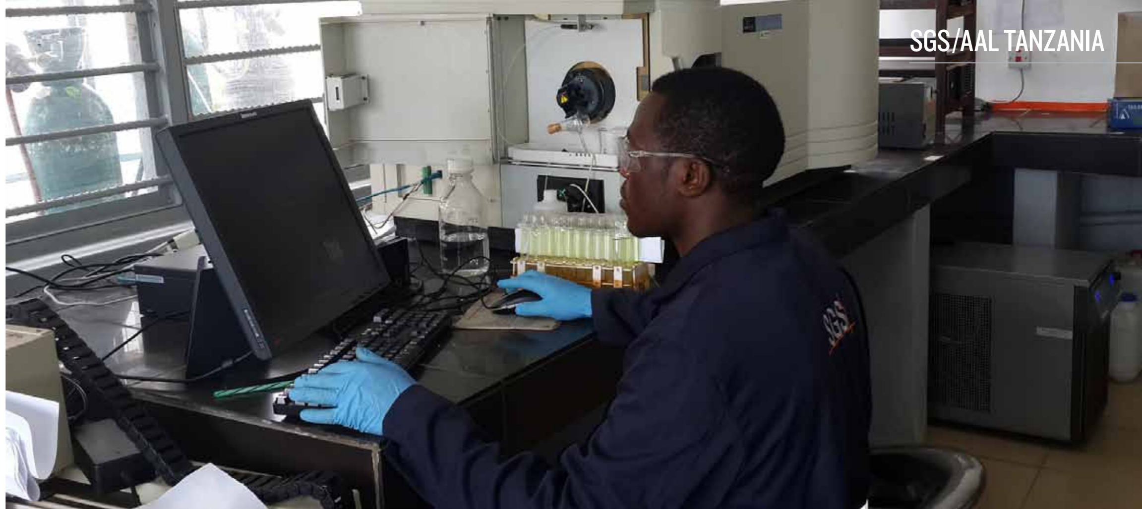
Chemist on ICP OES for determination of base metals in rocks & soils
