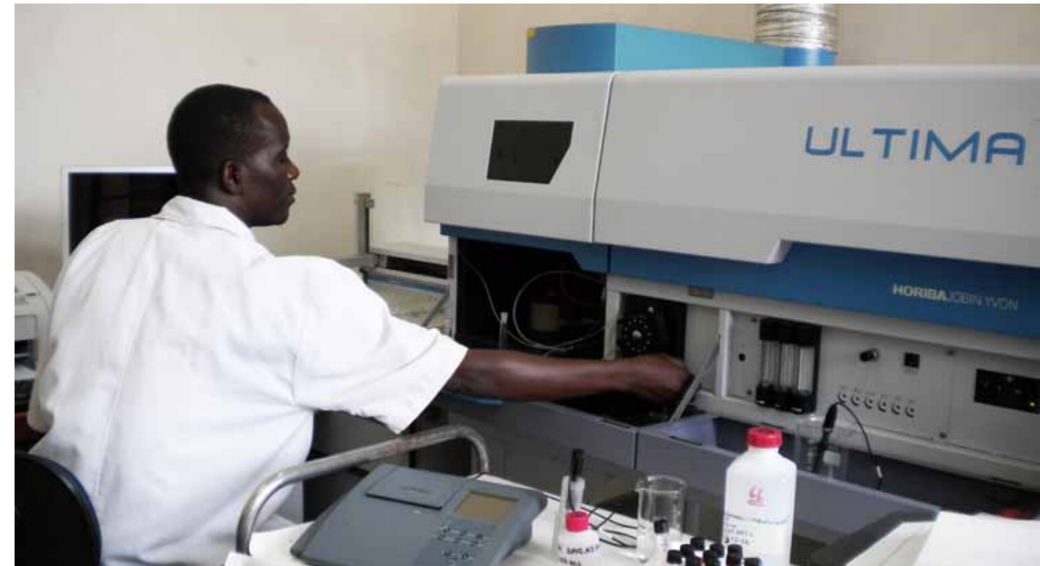
Environmental samples Analysis using Inductively Coupled Plasma (ICP) technique
