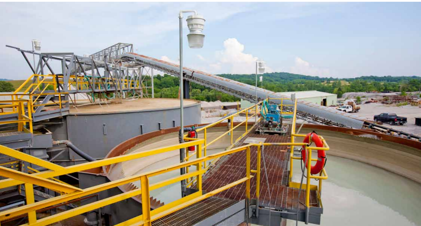
A pair of thickening tanks at the Middle Tennessee mill, with the conveyer belt that routes the agricultural lime to its storage area
