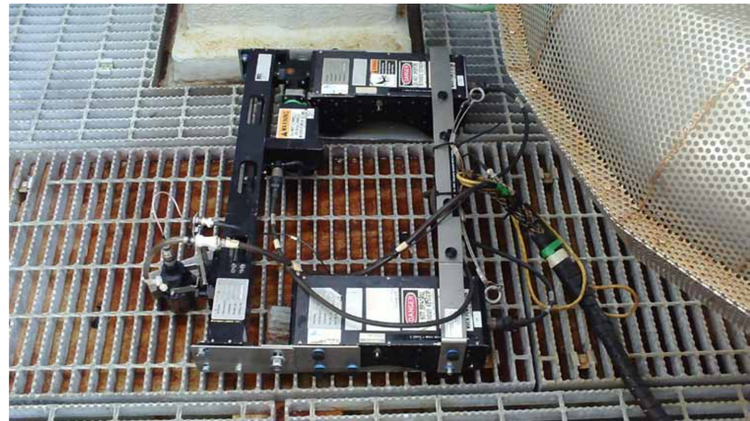
A robotic scanner operated via umbilical cable can map at rates of 15 – 150 square metres per day
