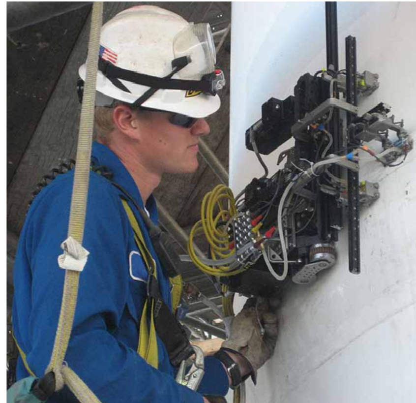
A weld scanner identifies cracking and corrosion in welds
