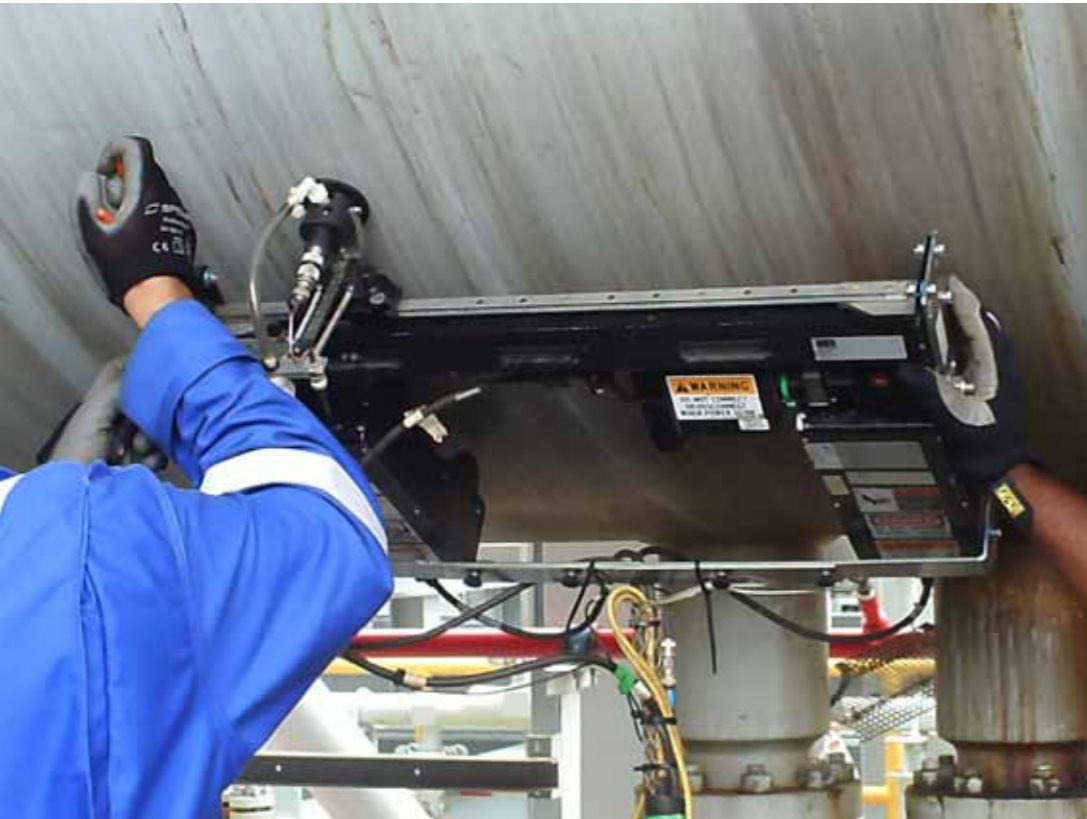
Final adjustments prior to launching a mapping scanner
