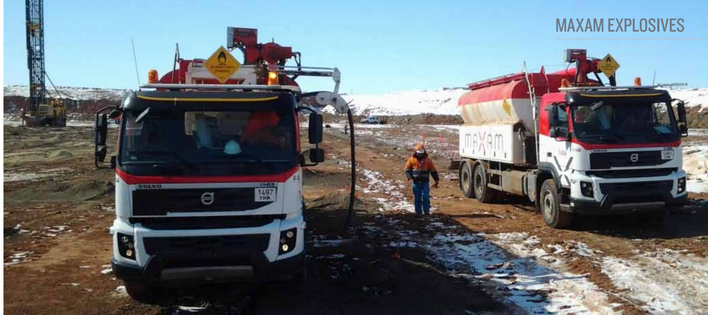
MAXAM’s latest mobile sensitising units delivering (MSUs) Rioflex 7000 at Oyu Tolgoi
