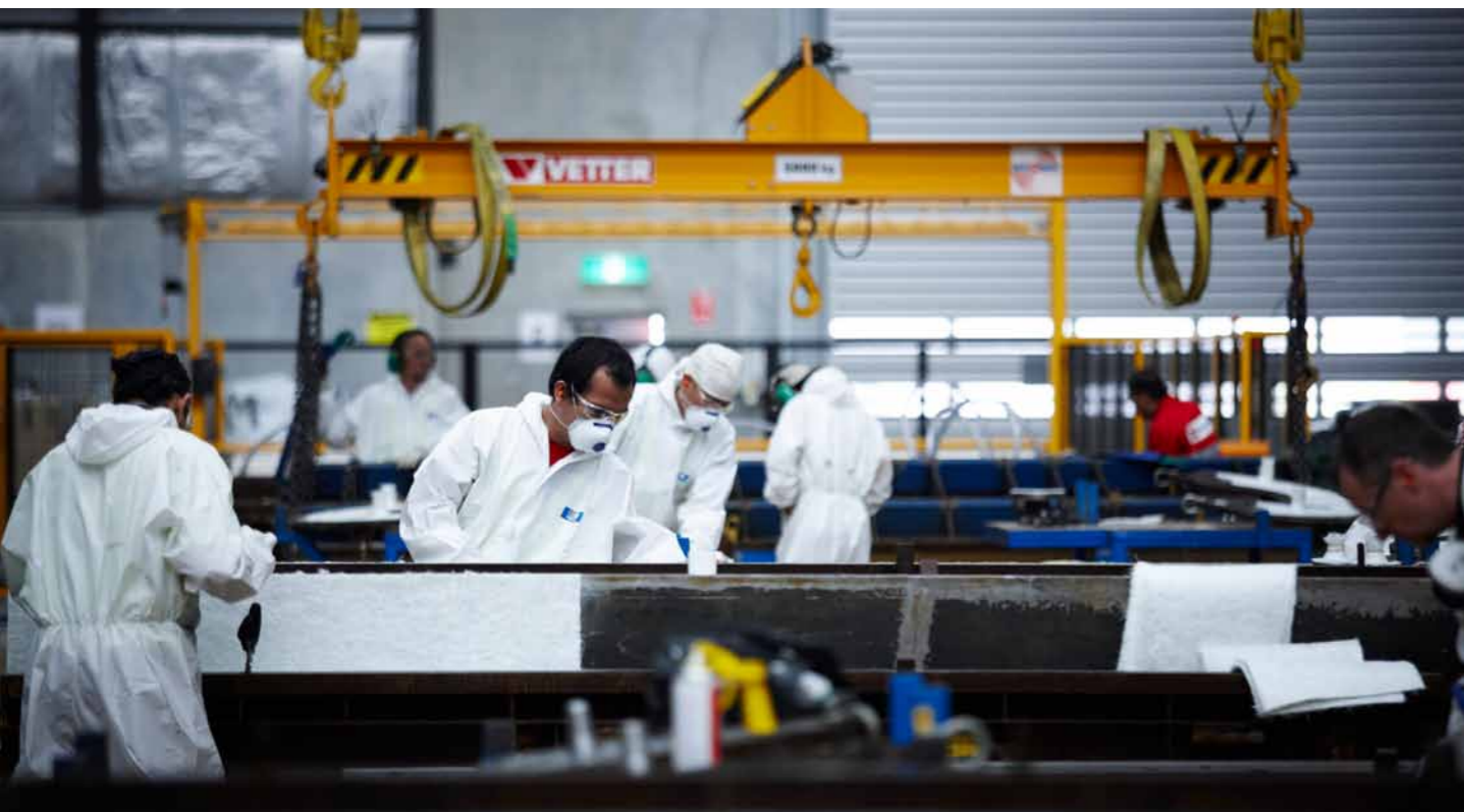
Matrix employees making buoyancy modules
