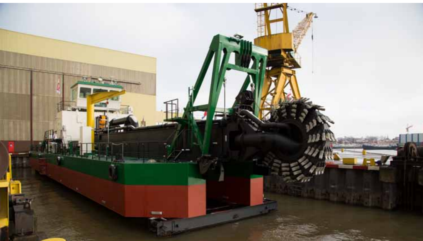
Dredge equipment for overburden removal
