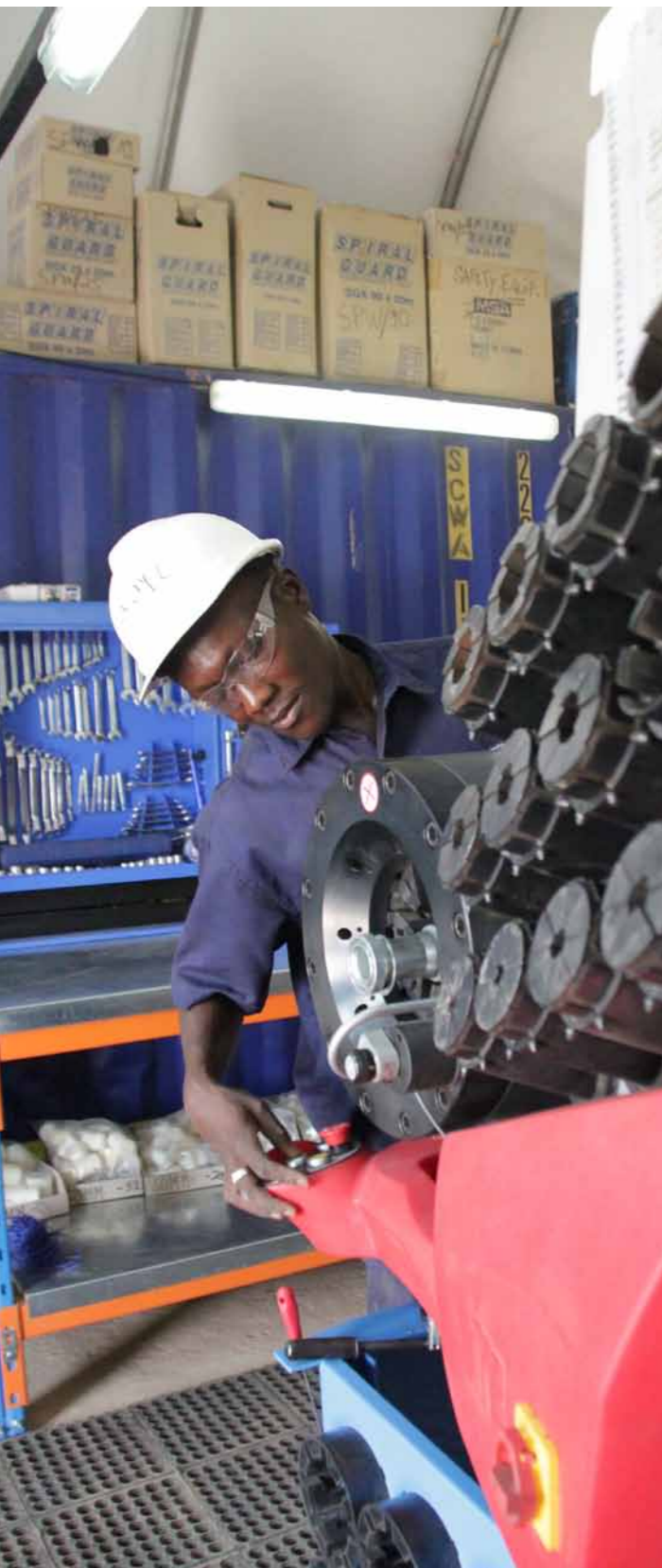
Hose crimping on site
