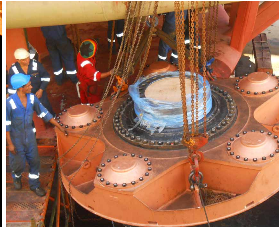
Refitting of Voith rotor into Enseleni Harbour tug
