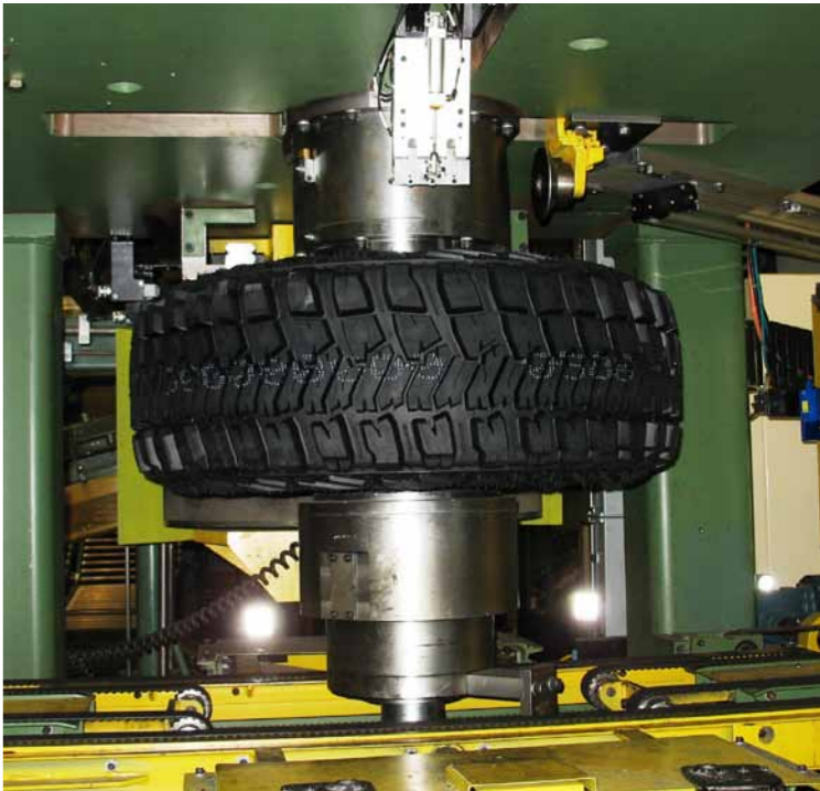
A tire going through a “test” drive in the Final Finish Dept
