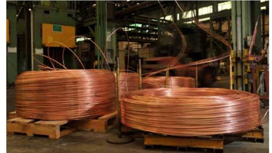
Elsewhere inside its facility bare, tin and nickel plated wires drawn by the company's drawing machine group are wound onto steel or plastic reels, before being reduced in diameter to between 0.05 millimetres and
