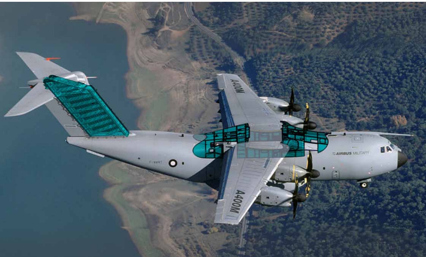
Denel Aerostructures is involved in three work packages for the A400M, the top shells, ribs swords and spars and the wing to fuselage fairing
