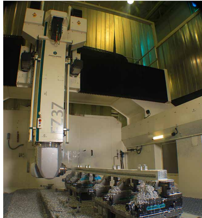
Denel Aerostructures specialises in advanced manufacturing. Two in house Zimmermanns allow for expertise in thin web machining
