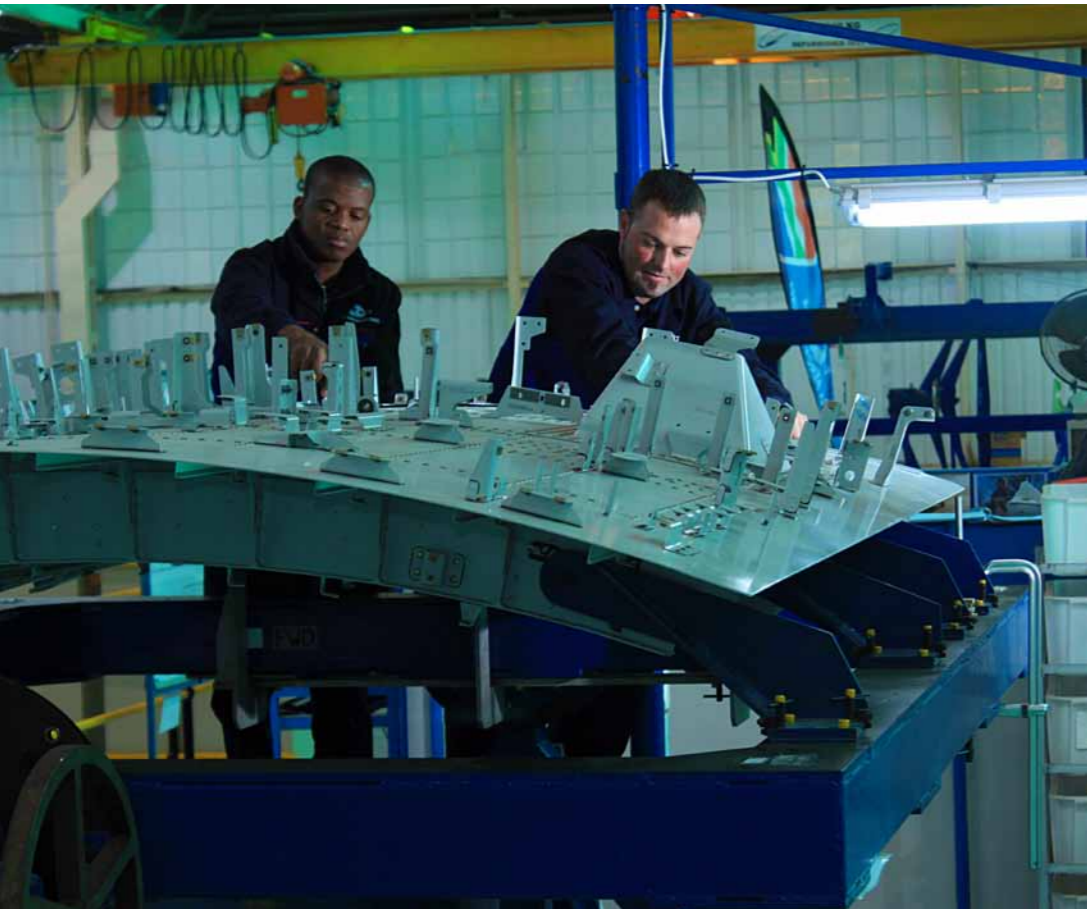
Denel Aerostructures' world class capabilities include an assembly line; above is the top shell assembly
