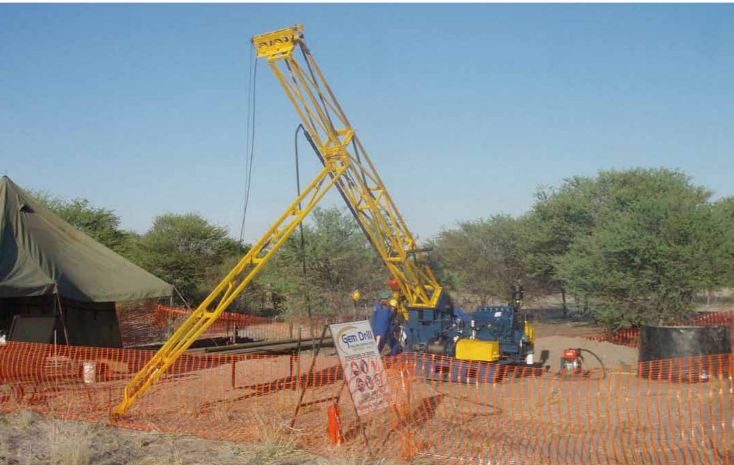
Gem Drill site: exploration drilling for diamonds
