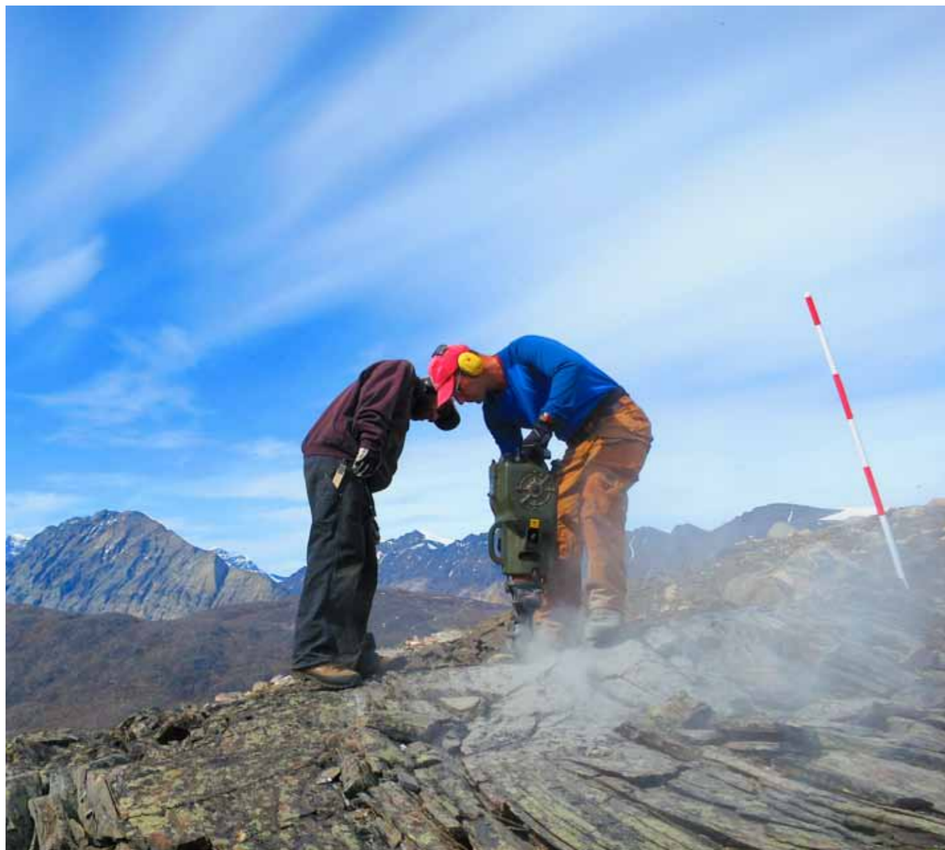
Drilling charge holes for a seismic survey in West Greenland where Avannaq is using seismic work in combination with other geophysical methods to constrain buried copper-nickel-PGE targets
