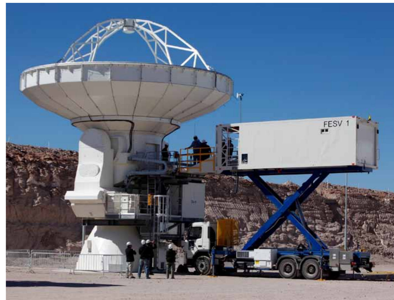
The Front End Service Vehicle in its raised position servicing the receiver cabin
