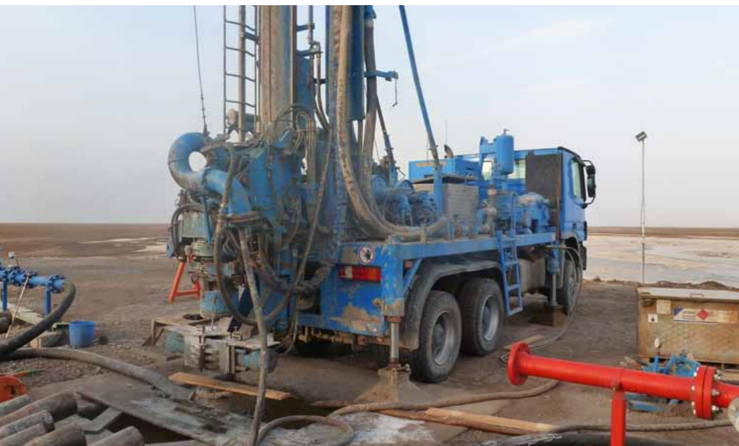
NBB water well and solution well drilling with nordmeyer drill rig
