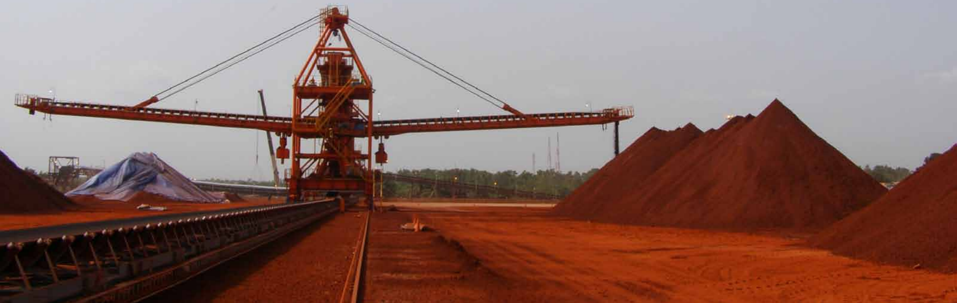
Reclaimer at work
